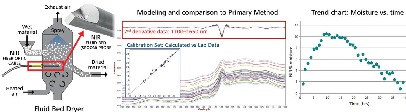
*Suggested placement for NIR “spoon” probe in a fluid bed dryer. Raw spectra of the dryer samples shows strong water absorption around 1400 nm, which is very evident in the 2<sup>nd</sup> derivative spectra. The 2<sup>nd</sup> derivative intensity (1100–1650 nm) was used to create a prediction model.*
